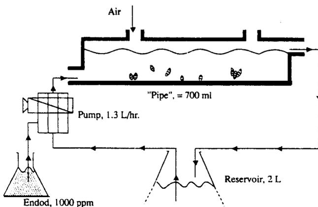
Figure 1. A recirculating system in which mussels were treated with Endod. Results of experiments using this system are shown in Tables 4 and 5.
